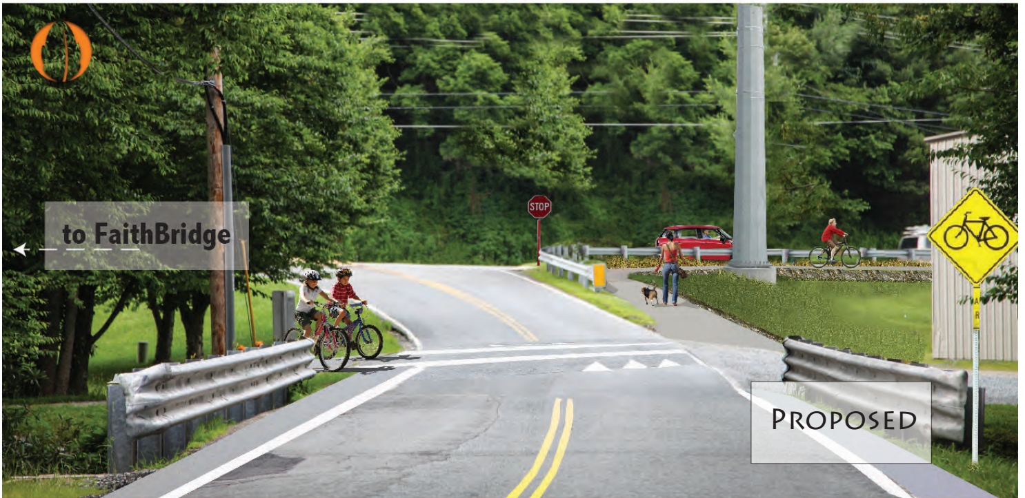
↗ A MARKED CROSSING AT AHO ROAD JUST BEFORE THE INTERSECTION WITH HIGHWAY 321. THE TRAIL THEN CONTINUES ALONG HIGHWAY 321 IN THE D.O.T. RIGHT-OF-WAY. THE EXISTING PINE TREES (RIGHT OF AHO ROAD) WILL NEED TO BE REMOVED TO INCREASE VISIBILITY AND ACCOMMODATE THE TRAIL. A LOW RETAINING WALL MAY BE NEEDED TO ENSURE A LEVEL TRAIL.
